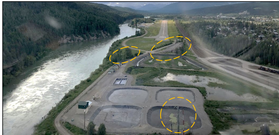
Obstacles under the Runway 32 approach, including the powerline, granular stockpile, and trees
