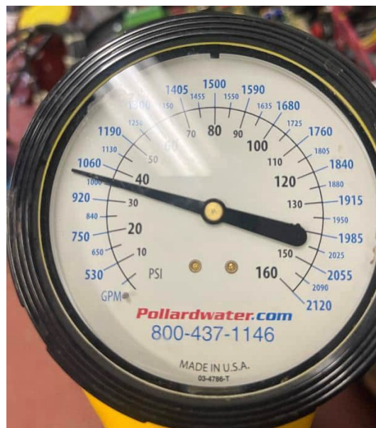
Figure 1. Gauge Used During Hydrant Testing at Atmospheric Pressure, Shows the Needle is Above Zero
